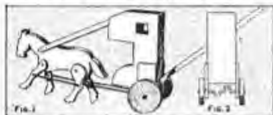
The Toy is Pushed by Means of the Handle, Causing the Horse to Walk
